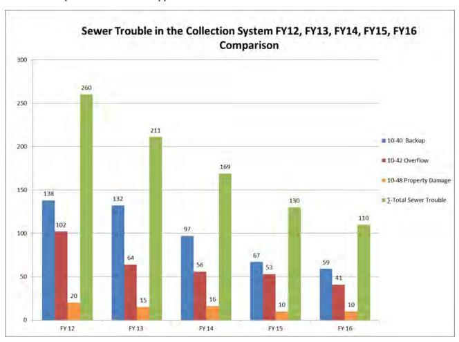
**Figure 2 Sewer Trouble Comparison**
