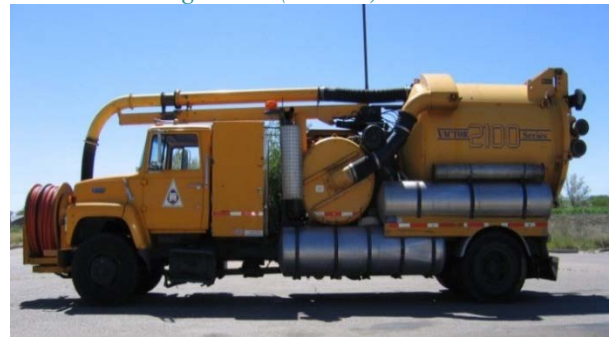
Sewer Cleaning Truck (Vactor)
