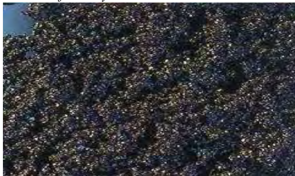
Granular ferric hydroxide arsenic removal media
