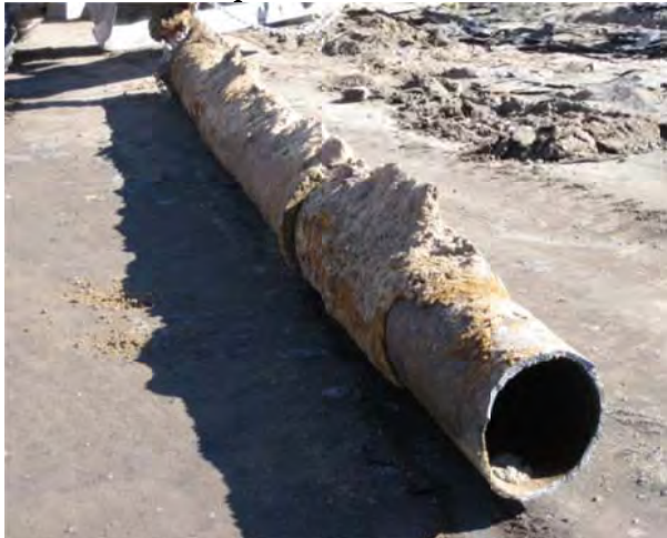
Corroded Steel Pipe
