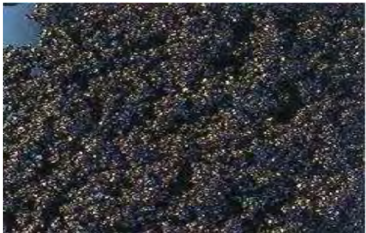
Granular ferric hydroxide arsenic removal media
