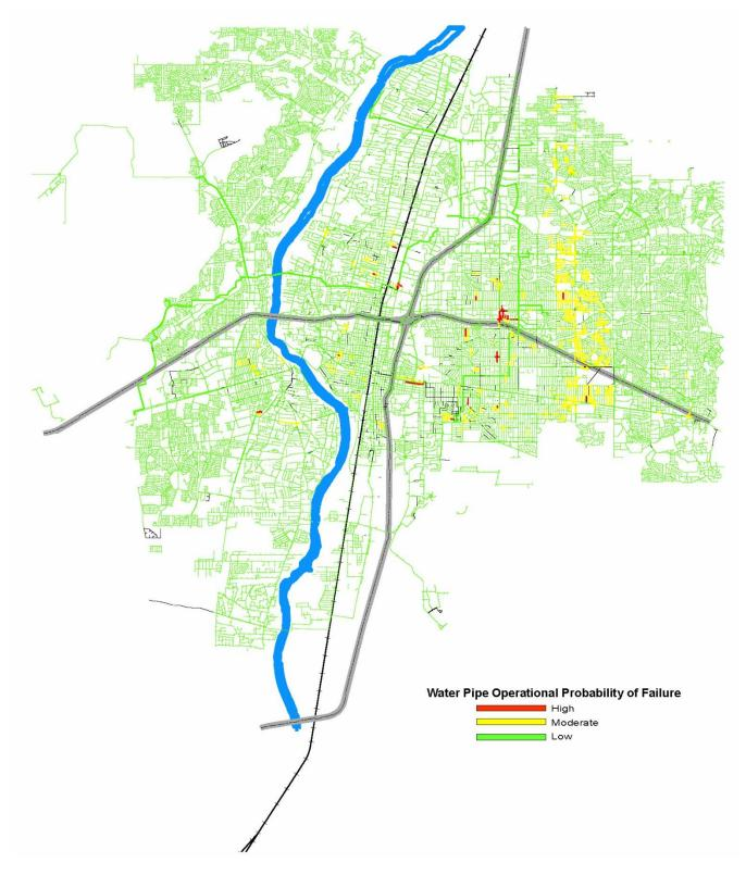
Figure 6-10 Water Pipe Operational Probability of Failure Results
