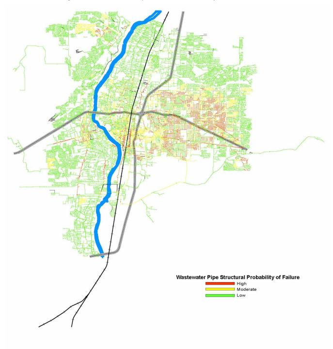
Figure 6-4 Wastewater Pipe Structural Probability of Failure Results
