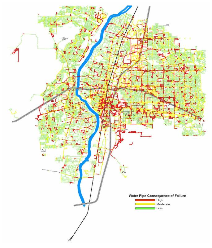
Figure 6-11 Water Pipe Consequence of Failure Results
