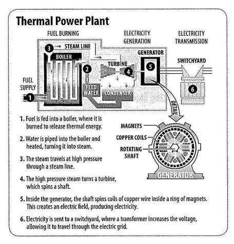
Thermal power plants can also use uranium to heat the water that makes steam that spins the copper wires. Uranium does not have energy from the sun. It is a radioactive metal found in the earth's crust. The nucleus of uranium is so large that it can be split into lighter elements, a process called fission. Fission gives off heat and other energy. The heat is used to boil water.
