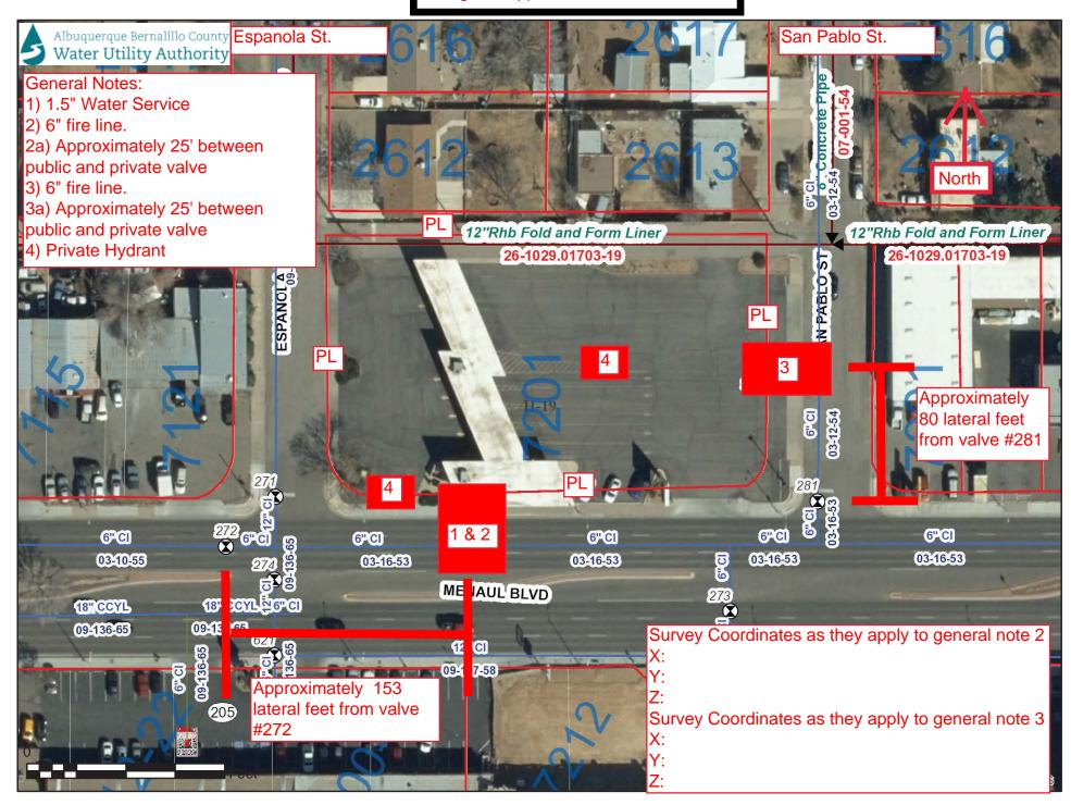
Valves needed for shut off
